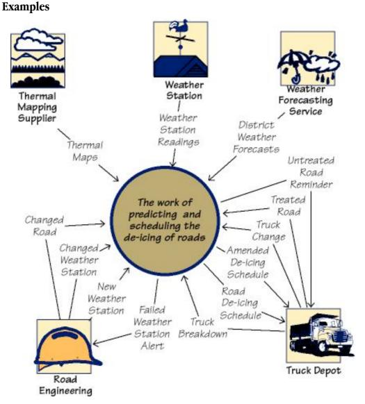
This work context model defines the connections between the part of the world that is under investigation and other people, organizations, hardware and software (referred to as adjacent systems). The inputs and outputs represent the data and material that travels between the work and other parts
